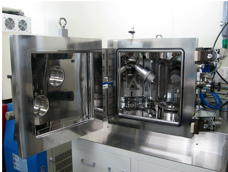
DLC Coating Chamber
